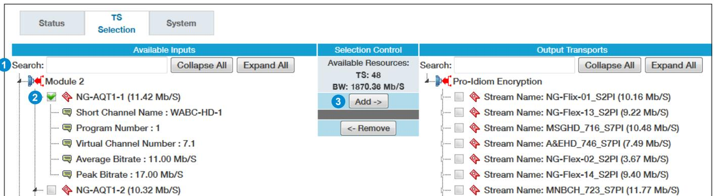
Figure 4.2 - “Transport Stream” Tab - Adding Programs
