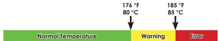
Figure 3.1c - Decoder Temperature Status Range
