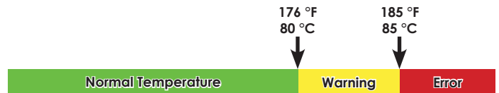
Figure 3.1c - Transcoder Temperature Status Range
