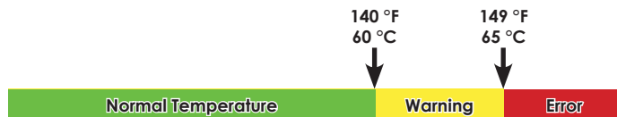
Figure 4.1b - Module Temperature Status Range
