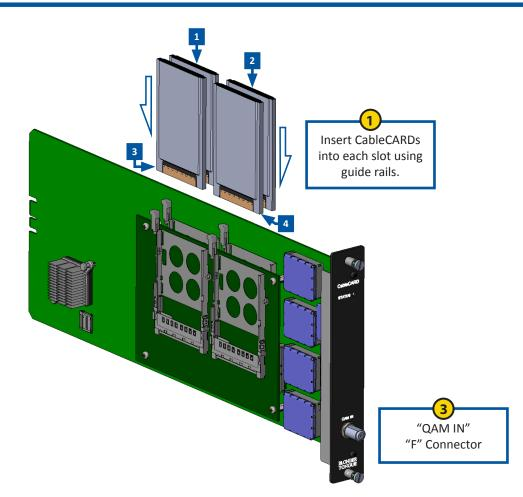
Install the CableCARD module into and empty slot on the NeXgen Gateway Chassis and secure with screws.
