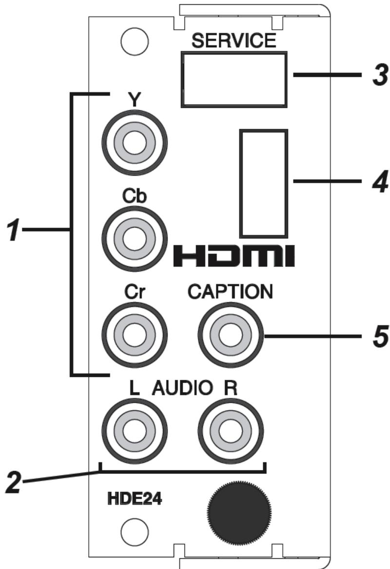
**1:** Component video input. Y input is used for Composite video input as well.
