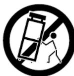
A product and cart combination should be moved with care. Quick stops, excessive force and uneven surfaces may cause the product and cart combination to overturn.
