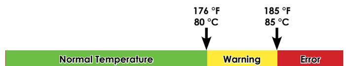
Figure 5.1b - Encoder Temperature Status Range
