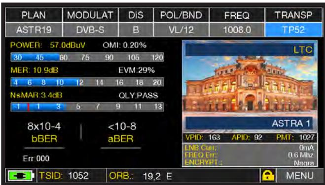
Main measurements and image of a SAT signal.
