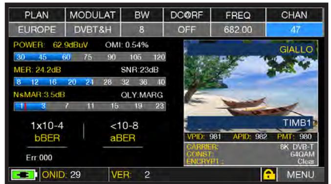
Main measurements and image of a TV signal.
