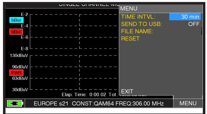
Select the time interval (TIME INTVL) and where you want to store the file, either in the meter's memory, or in the USB memory stick (Send to USB - ON), with the relative File Name.
