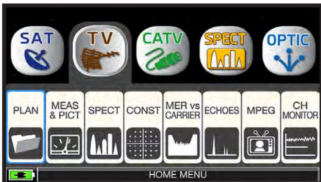
Touch "TV" and then "PLAN" or use the wheel to access the TV channel plan list.
