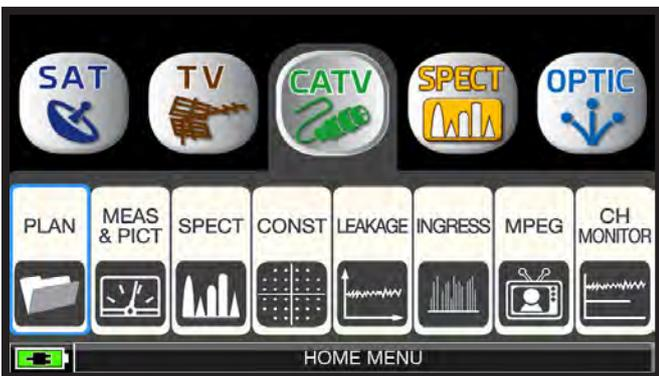
Touch "CATV" and then "PLAN" or use the wheel to access the CATV channel plan list.
