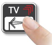
Press repeatedly to navigate into TV measurements screens: Measurements, Constellation, Echoes and MER vs CARRIER.
