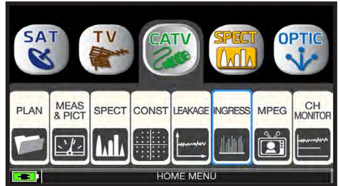
Touch "CATV" and then "LEAKAGE" or use the wheel.
