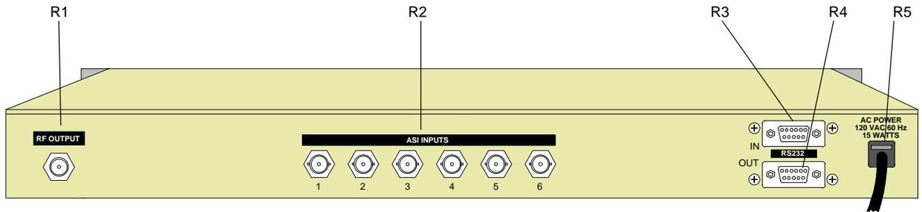
**R1, RF OUTPUT** – This type "F" connector is the high level (+40 dBmV), 54 to 1002 MHz, output from the MQM6000L upconverter section.
