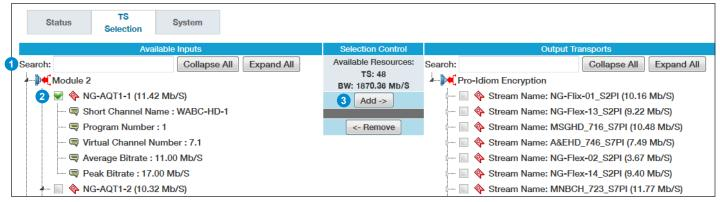
Figure 4.2 - "Transport Stream" Tab - Adding Programs
