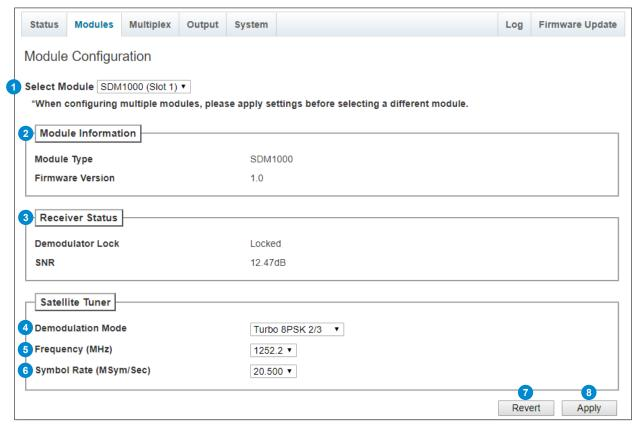
Figure 4.2 - "Modules" Tab - Module Configuration
