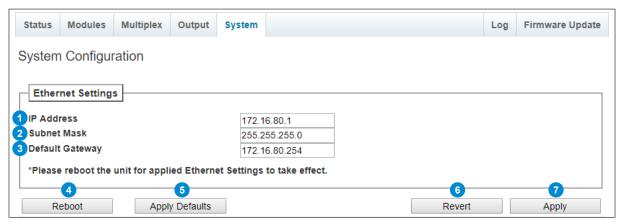
Figure 5.1 - "System" Tab - System Configuration
