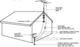
NEC - NATIONAL ELECTRIC CODE Example of antenna grounding as per National Electrical Code, ANSI/NFPA 70
