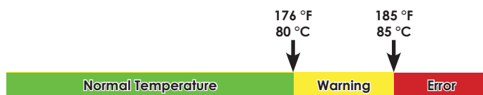
Figure 5.1b - Decoder Temperature Status Range
