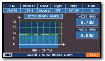
Buzzer & Graphic of the progress of the noise NOISE MARGIN of the tuned channel according to time.
