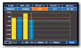
Touch "PILOT 1" and "PILOT 2" to select the two channels to be used for the tilt measurement (level difference)
