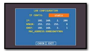
Touch "IP CONFIG" and select "STATIC", insert the "IP" parameters, "NMASK" & "GWAY"
