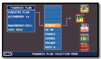
In TV or CATV mode press the "PLAN" key, select the plan required, then "SPECT" to visualize the spectrum
