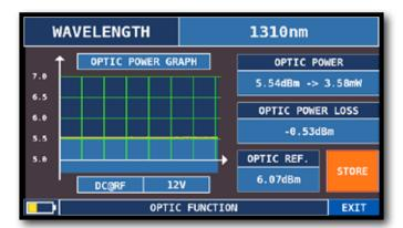
The "OPTIC POWER LOSS" field shows the optical attenuation value compared to the stored value (Optic REF): for example: - 0,53 dBm
