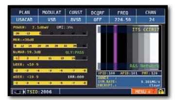
Press the "TV" key to carry out the RF measurements & OMI
