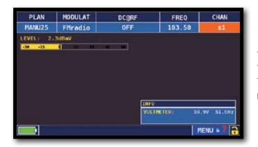
Touch "CHAN" & select "FMH" or "FML", Touch "MODULAT" & select "FM Radio", Touch "FREQ" and select the frequency required.
