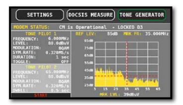
The meter is capable to send different tones at a well-determined level in order to detect the overall attenuation due to all the network elements (cables, routers, connections, ...) between the measurement point and the CMTS.
