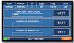
The "HELP" function will try to identify the tuning parameters of the selected digital carrier
