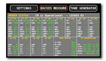
The meter will start scanning the selected channels in order to connect to the CMTS While performing this process the display will indicate <u>Scanning now</u> at bottom and <u>WAIT</u> or <u>UNLOCKED</u> in the various parameters fields. Once completed the synchronization process, the LCD will display "CM is Registered" and will report a summary of the major information about the active connection:
