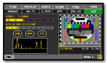
Level measurement, audio-vidio measurement and picture
