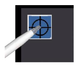
NOTE: Use the pen and touch the screen exactly in the center of the circle. if you do not carry out this procedure correctly the touch commands may be inaccurate.
