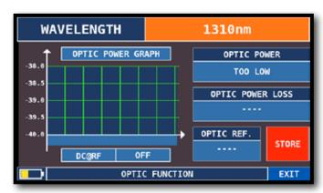
Touch "WAVELENGTH" and select the required wavelength, for example 1310 nm
