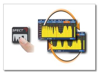
Press to cycle through spectrum analyzer screens
