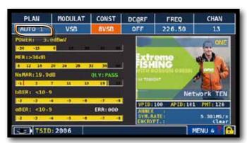
Upon automemory completion the new plan is automatically selected
